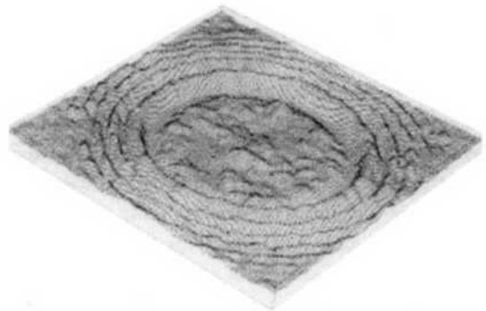
(b) Intensity modulation of interferogram by monochromatic incident light under Hertzian contact condition (5 N static load)
